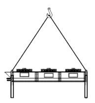
If the desired angle cannot be provided with a single rope mechanism in the product, transportation should be done with the equipment in the visual.
