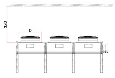
• When placing the product, a distance of at least the support legs clearance (H) should be left on all four sides to ensure unobstructed air flow and comfortable maintenance, cleaning and repair conditions.
