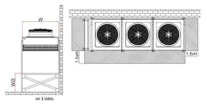
• If there is a certain opening between the wall and the product, it is useful to close it as shown in the figure below so that the air flow does not bypass.
