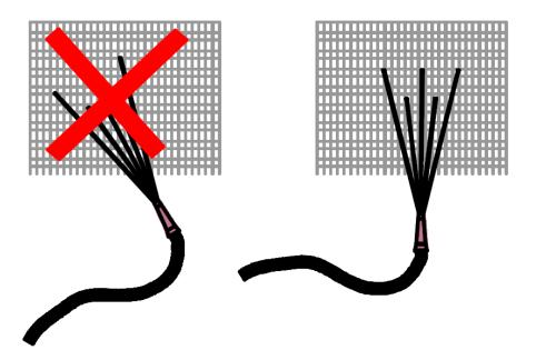
(\*) In order to prevent damage to the fin surface, water should be held at a right angle while washing with water.
