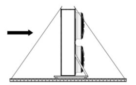
If there is no wall to support the product, the product should be secured using a rope device and flag.
